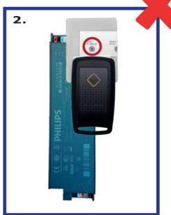
For optimal reading of LED drivers using NFC Passive Repeater, the reader must be positioned in "edge reading" over the NFC area of LED driver, in correspondence with "Focus 2" on the label, or sideways from the NFC area logo, as shown in figure 1.
