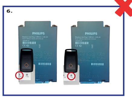
For optimal reading of LED drivers using NFC Passive Repeater, the reader must be positioned sideways from the NFC area logo, as shown in figure 5.
