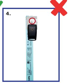
For optimal reading of LED drivers using NFC Passive Repeater, the reader must be positioned in "edge reading" over the NFC area of LED driver, in correspondence with "Focus 2" on the label, or sideways from the NFC area logo, as shown in figure 3.
