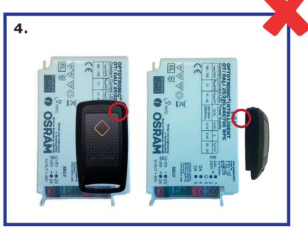
As regards the optimal reading of OTI DALI LED drivers, NFC Scanner must be positioned in "center reading" over the NFC area of LED driver as shown in figure 3.
