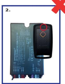
As regards the optimal reading of the OT LED drivers, NFC Scanner must be positioned in "edge reading" over the NFC area of LED driver or sideways as shown in figure 1.
